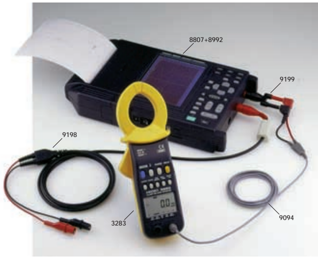
For long-term monitoring, use the Model 9418-10 AC ADAPTER for the 8807-01 MEMORY RECORDER and the Model 9445-02/03 AC ADAPTER for the 3283 CLAMP ON LEAK HITESTER
