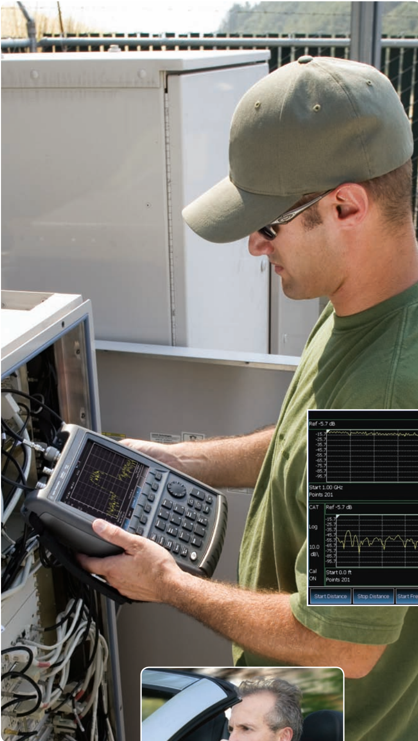
Return loss and DTF dual display
