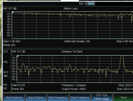
Return loss and DTF dual display
