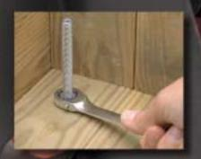
This wrench works in places even deep sockets won't reach. It's perfect for positioning and tightening bolts on threaded rods.
