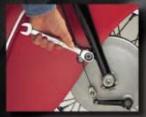
The 15° offset makes it possible to tighten fasteners while keeping the wrench safely away from easily scratched surfaces.
