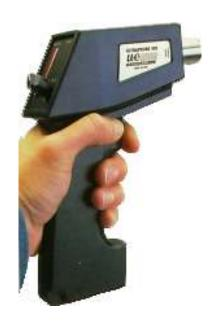
The Ultraprobe senses high frequency sounds produced by operating equipment, leaks and electrical discharges. It electronically translates these signals by heterodyning them down into the audible range so that a user can hear these sounds through a headset and see them as intensity increments on the meter. Heterodyning works the same as a radio in that it accurately transforms the sounds so that they are easily recognized and understood.
