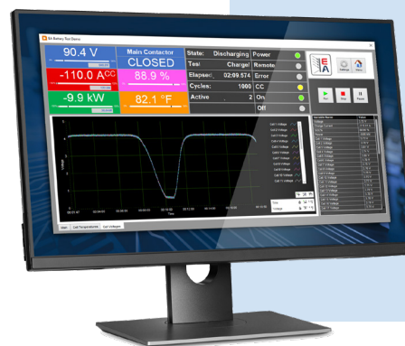
Results display screen showing voltage, current, and the results of a capacity simulation test.
