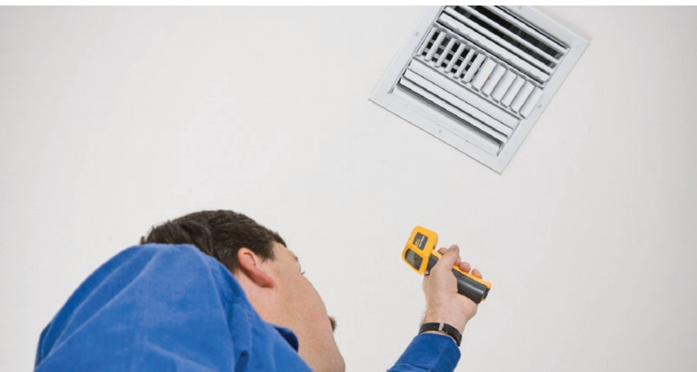
Use non-contact temperature measurements for inaccessible targets.
