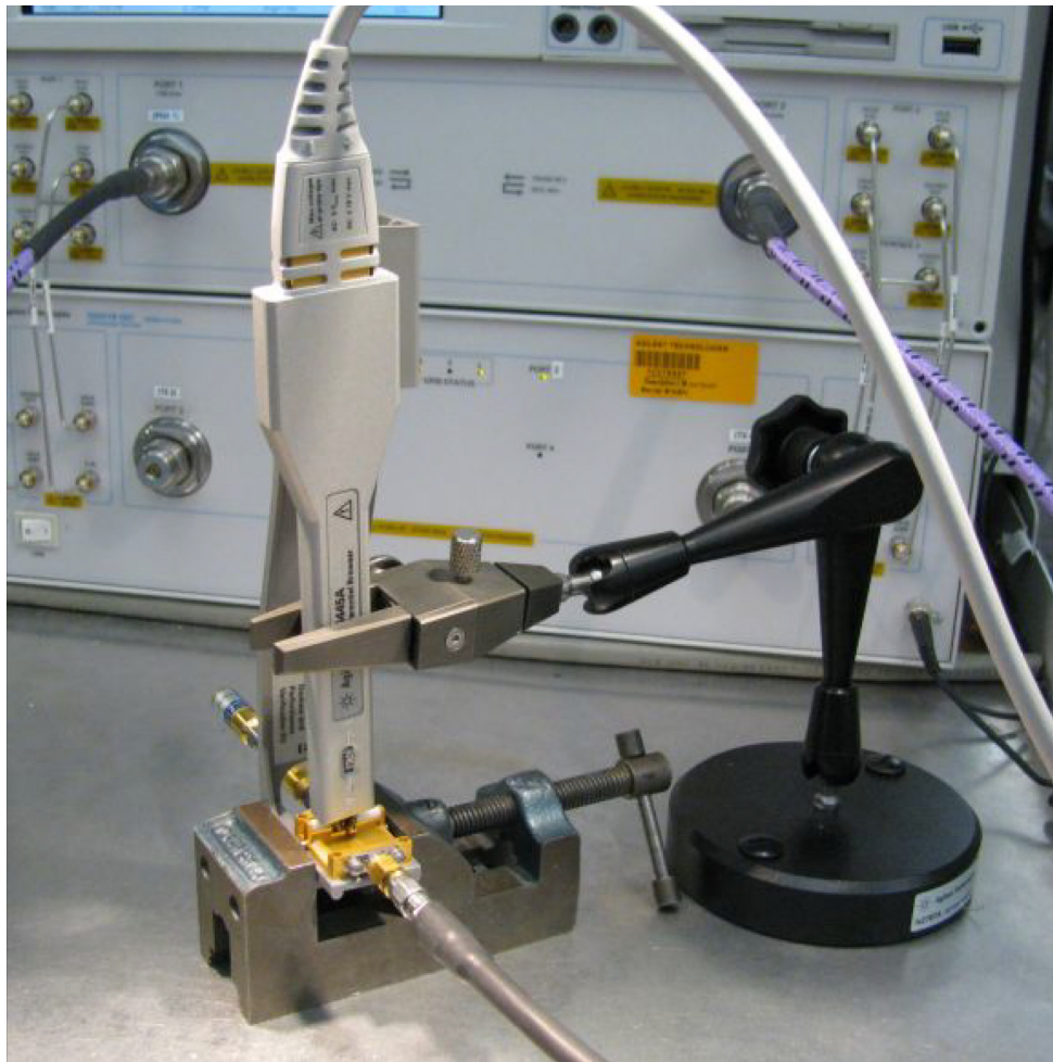
Figure 69 N2787A 3D Probe Positioner used to measure the N5445A browser with the N2803A amp
