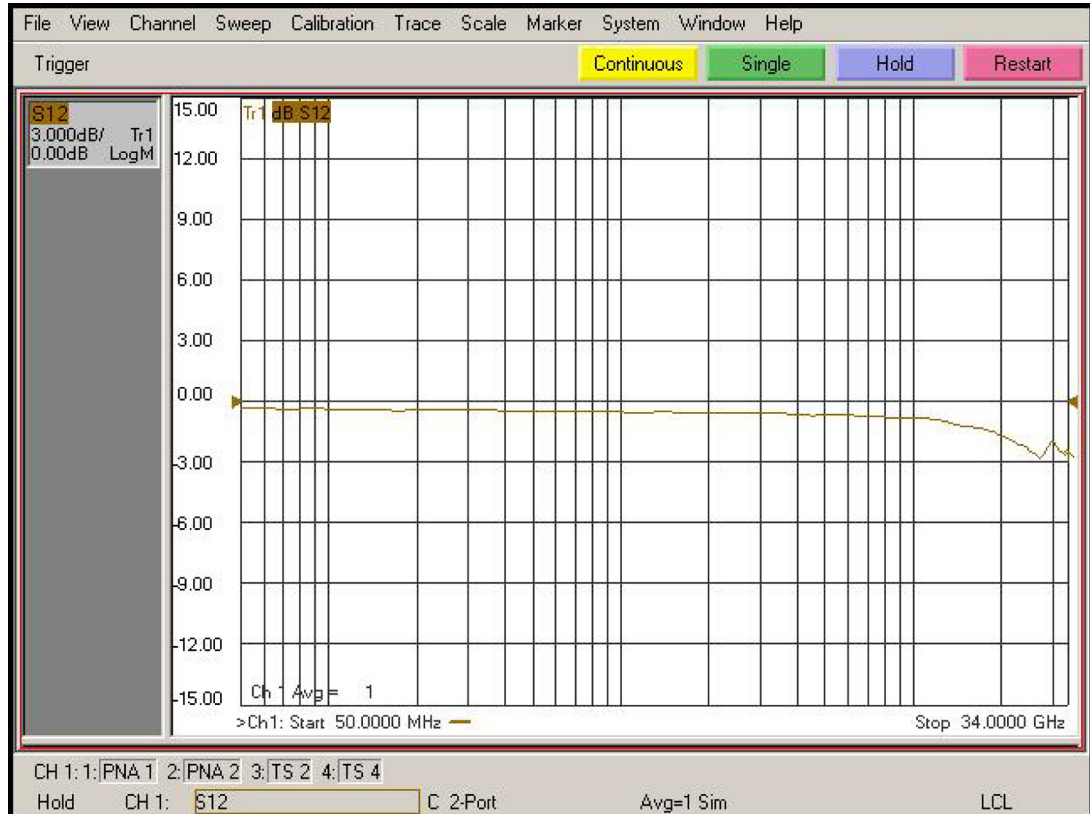
Figure 64 De-embedded “Vin” trace
