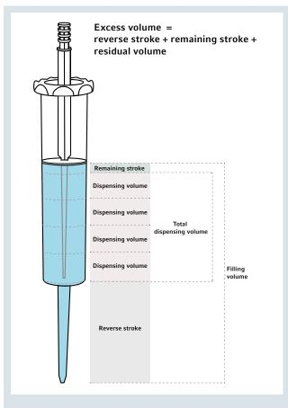
Figure 1: Stepwise distribution of filling volume
