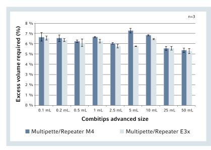
**Figure 2:** Excess volume required for complete filling of the Combitips advanced using Multipette/Repeater M4 or Multipette/Repeater E3x ranges between 5.3 and 6.7%.
