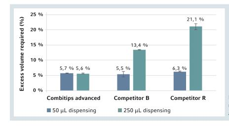
**Figure 3:** Excess volume for dispensing the nominal volume of 2.5 mL in Combitips advanced and two competitors dispenser tips. n=3
