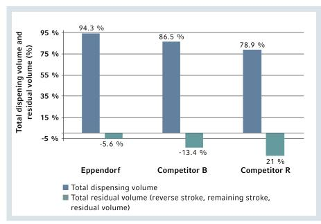
**Figure 4:** Dispensing volumes in 2.5 mL tips showing that competitor B and R have less total dispensing volume and more residual volume than Combitips advanced.
