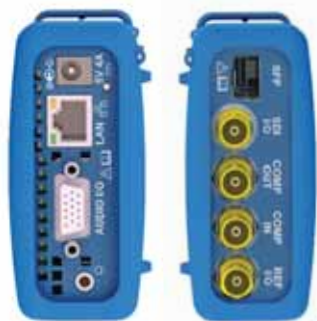
DC 5V power & recharge Ethernet Headphone D AES Composite In/Out, HD, SD SDI In or Out Bi/Tri-level Reference In/Out SFP cage
