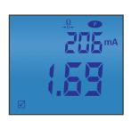
Continuity Measurement and test current Red Backlight and X indicates Alarm (Fail) Condition
