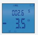
If the difference is below the programmed threshold, the symbol is displayed.
