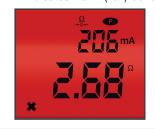
· At each new measurement, the instrument indicates the difference between the new reading and the reference measurement, along with the difference in %.
