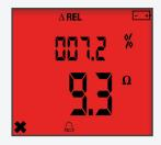
If the difference exceeds the programmed threshold, the X symbol is displayed and the backlight turns red.
