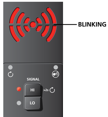
Figure 3.1b: Transmitter indicator showing signal in HIGH mode
