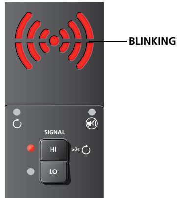
Figure 4.12b: Transmitter indicator showing signal in Loop mode
