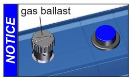
If pumping condensable vapors (water vapor, solvents, etc.), let the pump (MZ 1C) run with **gas ballast** to help purge any condensation in the pump.
