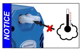
Avoid overheating (e.g., due to hot process gases). Maximum permissible temperature range: see "Gas inlet temperatures", pg. 24.
