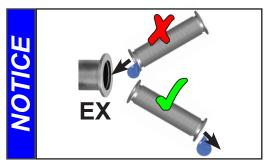
Always install outlet tubing descending from the pump or provide other measures to avoid backflow of condensate towards the pump.
