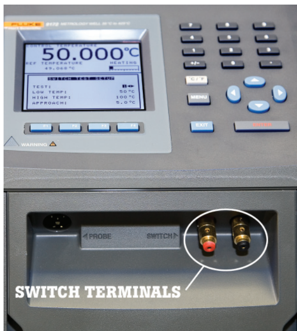
Figure 2 Location of the switch terminals on a Metrology Well.
