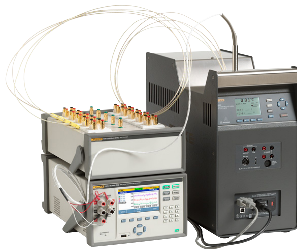
Fluke Calibration 1586A Super-DAQ Precision Temperature Scanner automates the calibration of thermocouples in a Fluke Calibration 9190A Ultra-Cool Field Metrology Well.
