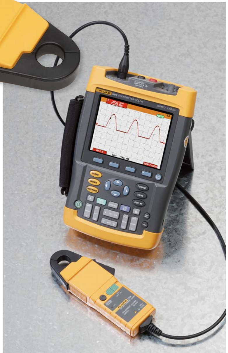
i30s connected to a Fluke 199C ScopeMeter™
