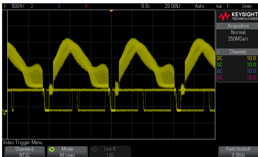
Figure 28 Triggering on All Lines
