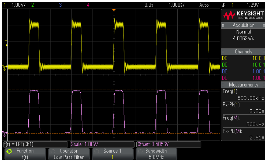
Figure 15 Example of Low Pass Filter
