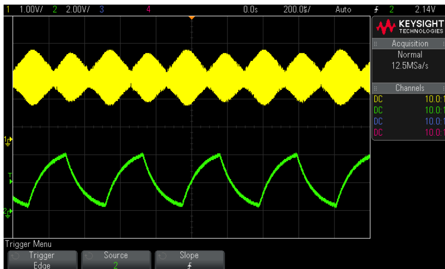
Figure 25 Amplitude Modulation Shown at 100% Intensity
