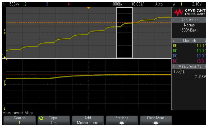
Figure 45 Isolating area for Top measurement
