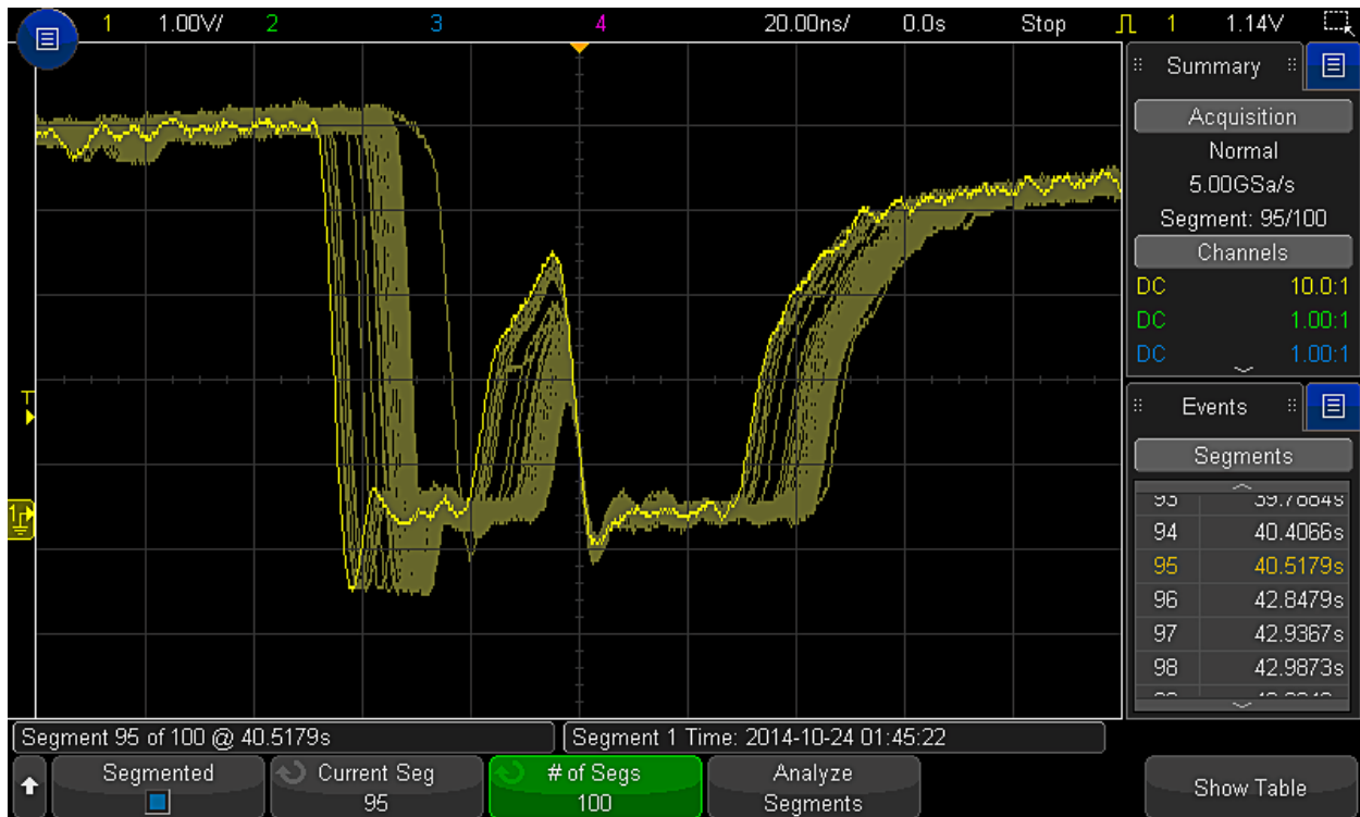
Figure 14. Screen showing an overlay of all 100 segments for worst case waveform analysis.
