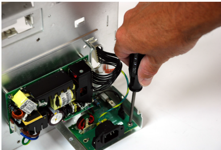
Figure 50 Removing the line filter board
