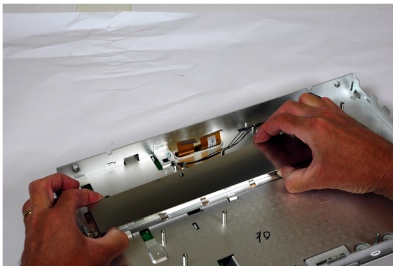
Figure 34 Removing the keyboard cable shield
