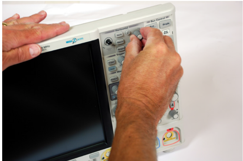
Figure 33 Removing the front panel knobs
