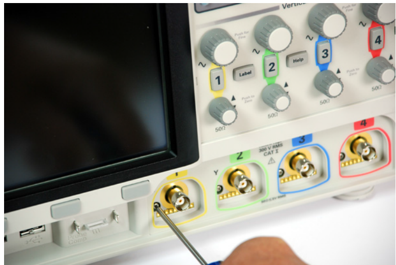
Figure 27 Removing the analog channel BNC securing T6 screws
