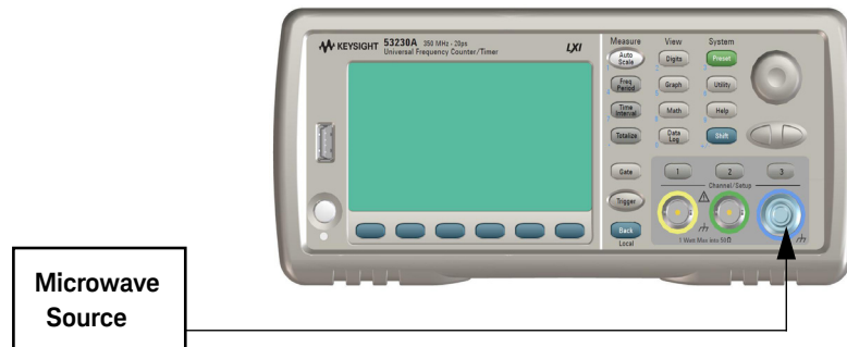
Figure 2-8 Microwave source connection to Channel 3
