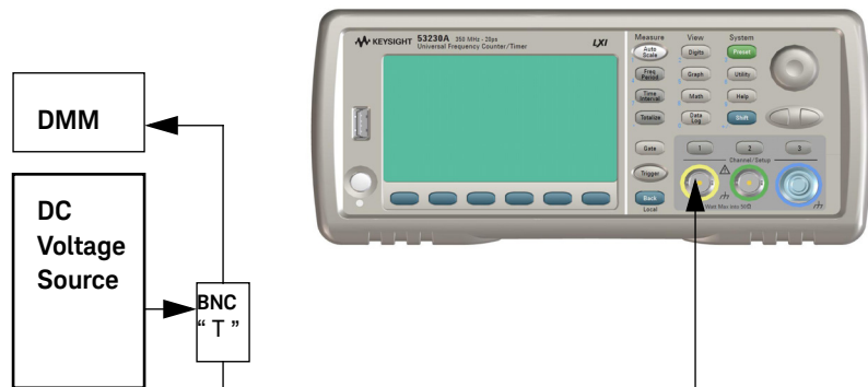
Figure 2-6 DC voltage source and DMM connections
