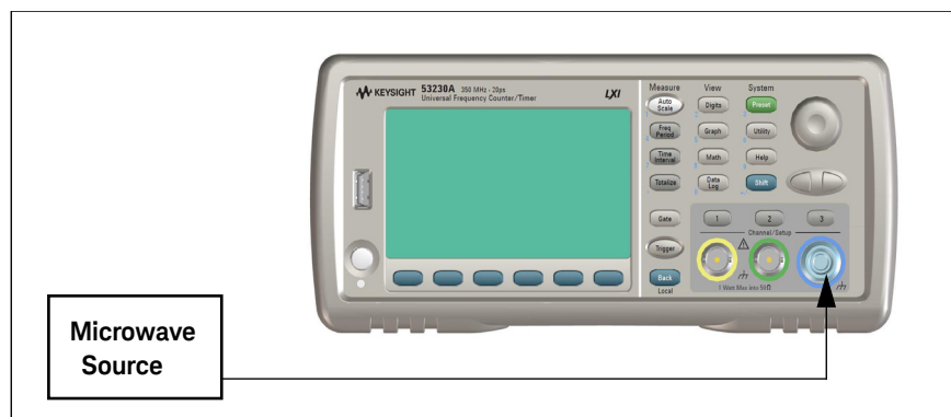
Figure 2-7 Microwave source connection to Channel 3
