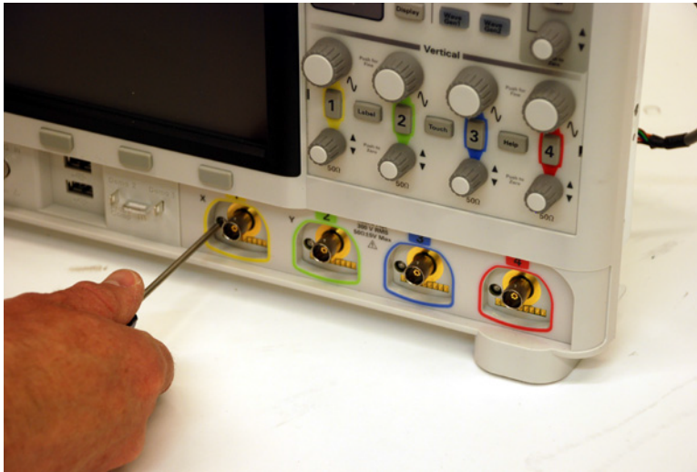
Figure 28 Removing the analog channel BNC securing T6 screws
