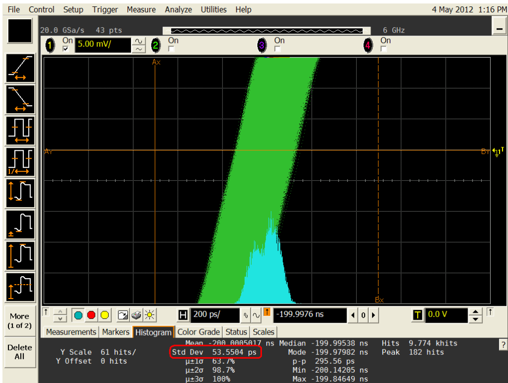
Figure 4. Jitter measurement on DDS signal.
