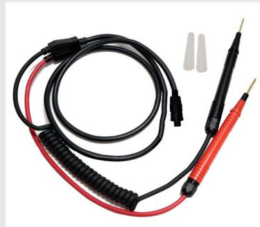
Connect the duplex probes to the BITE5 ADVANCED.
