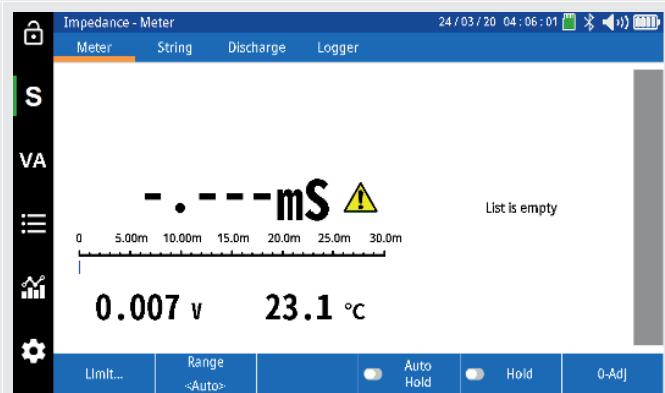
When the Siemens (S) ICON is selected the BITE5 Advanced will use the Duplex inputs.
