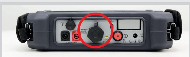
When the Ohm ( $\Omega$ ) ICON is selected the BITE5 Advanced will use the Duplex inputs.
