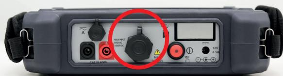
Connect the duplex probes to the BITE5 ADVANCED.
