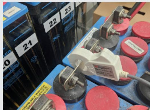
Continue taking measurements of each cell and strap in sequence until you reach the last cell in the string. When the BITE5 ADVANCED measures the last cell in the string, it will display a summary.
