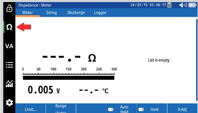
When the Ohm ( $\Omega$ ) ICON is selected the BITE5 Advanced will use the Duplex inputs.
