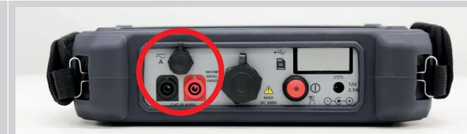
Connect the voltage leads to voltage inputs of the BITE5 ADVANCED.
