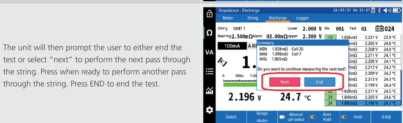
The unit will then prompt the user to either end the test or select "next" to perform the next pass through the string. Press when ready to perform another pass through the string. Press END to end the test.
