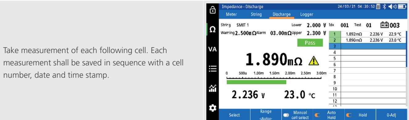
Take measurement of each following cell. Each measurement shall be saved in sequence with a cell number, date and time stamp.
