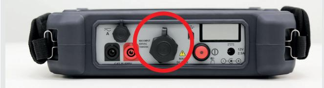
Connect the duplex probes to the BITE5 ADVANCED. to voltage inputs of the BITE5 ADVANCED.
