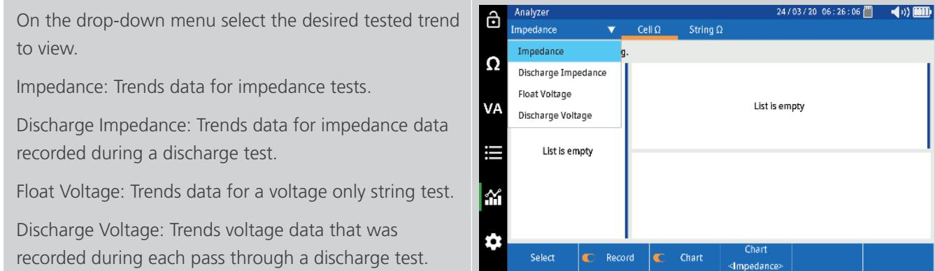
On the drop-down menu select the desired tested trend to view.
