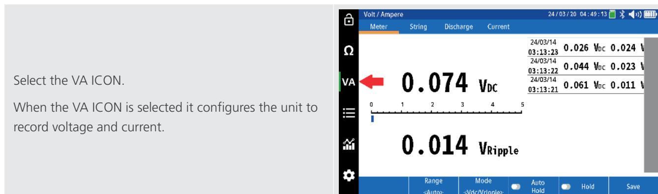
When the VA ICON is selected the BITE5 Advanced will use the banana jack inputs and the current clamp input. (if desired)
