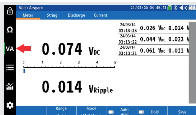
When the VA ICON is selected the BITE5 Advanced will use the banana jack inputs and the current clamp input. (if desired)
