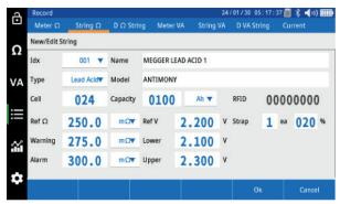
Impedance testing: measure cell impedance, cell voltage, cell temperature and strap resistance.
