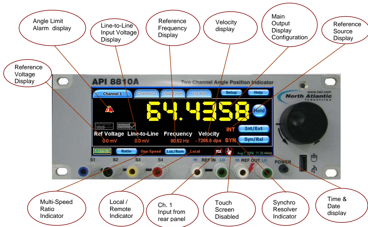
Figure 2 – Indicators on the front panel main display of the 8810A
