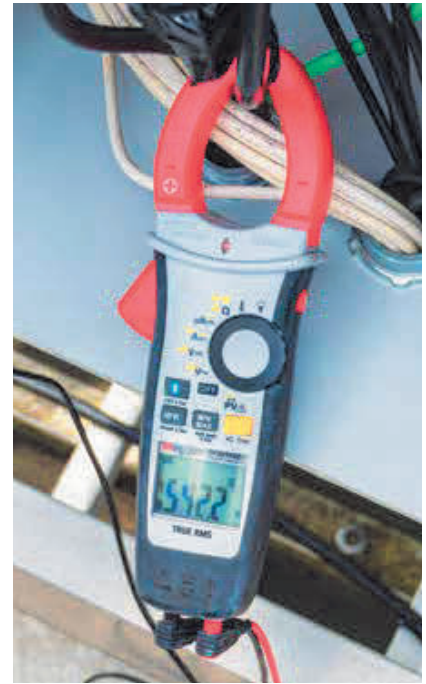
Figures 4-16 and 4-17: A field technician uses a DMM to confirm expected voltages and polarity in a PV combiner box.
