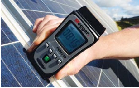
Figure 5-8: Irradiance is read with an irradiance meter placed on the same plane of the PV modules that are under testing. Technicians record the value and use it to calculate the actual current flow against the STC conditions.
