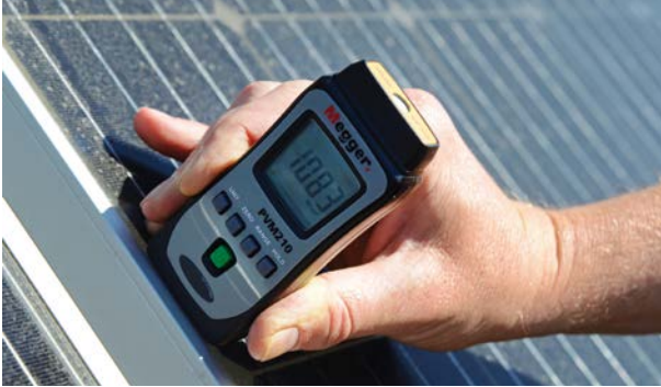
Figure 5-20: PV module current is directly proportional to the irradiance striking the module. The irradiance meter should be used at the same angle as the modules to improve measurement accuracy.
