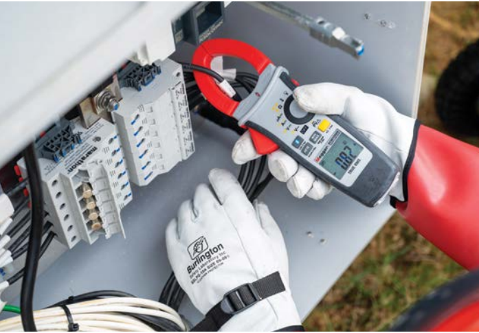
Figure 5-4: A clamp meter measures the current flowing through the conductor or bundle of conductors enclosed within the clamp.
