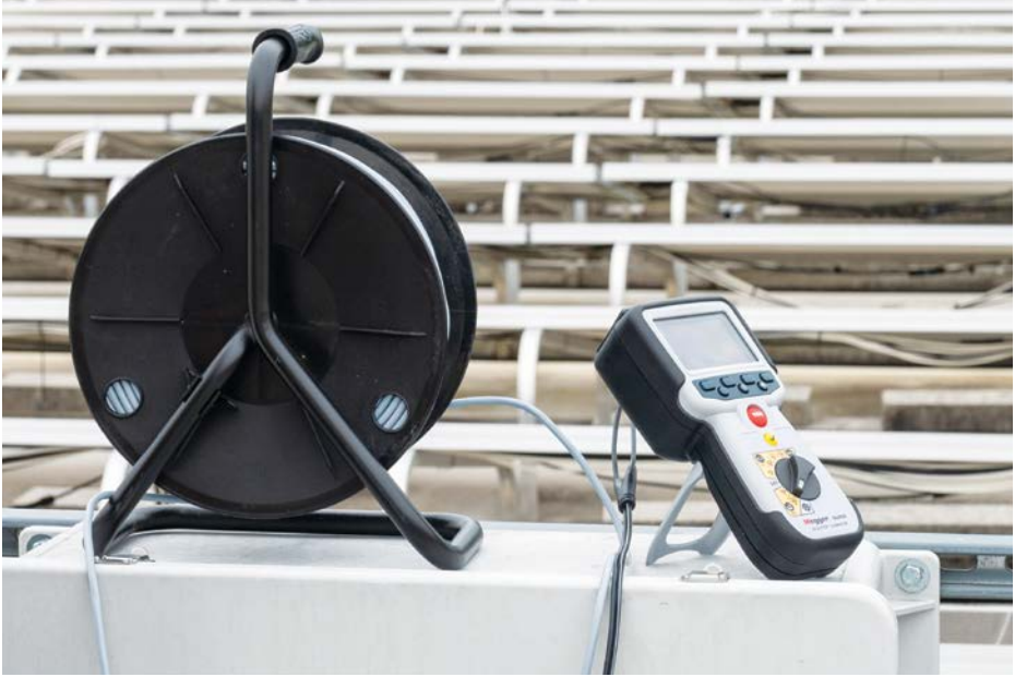
Figure 6-16: Meters with data storage can be utilized to document site readings and establish long term trends.
