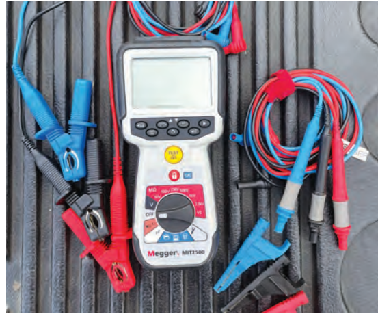
Typical insulation resistance test instrument and associated leads.
