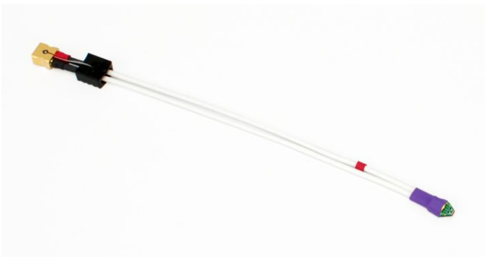
TriMode™ Long Reach Solder Tip (0 Ω tip resistor) A high performance solder tip for use with memory chip interposers with embedded 175 Ω resistors. Up to 20 GHz bandwidth.
